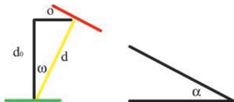
Fig. 2 Definition of the geometric parameters. Shown in yellow is the distance d between the centroid of the indole from Trp279 (green) and the centroid from the aromatic a-ring of galanthamine (red). The angle \alpha describes the angle between the two ring planes. \omega describes the angle between the normal on Trp279 and the distance vector. d_0 and o are parameters of interest for \pi - \pi interactions, the distance of the (assumed parallel) planes and the offset of the centroids within a plane
